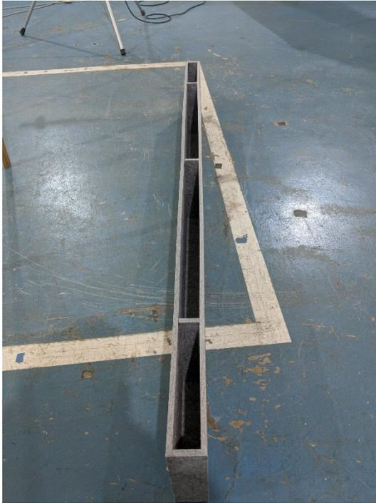
Figure 3 – Individual specimen object prior to mounting, hollow interior and support members
