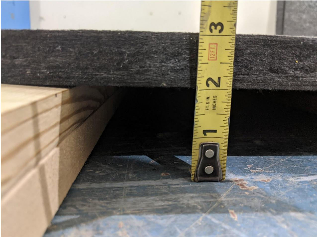
Figure 5 – Detail of specimen materials and airgap depth
