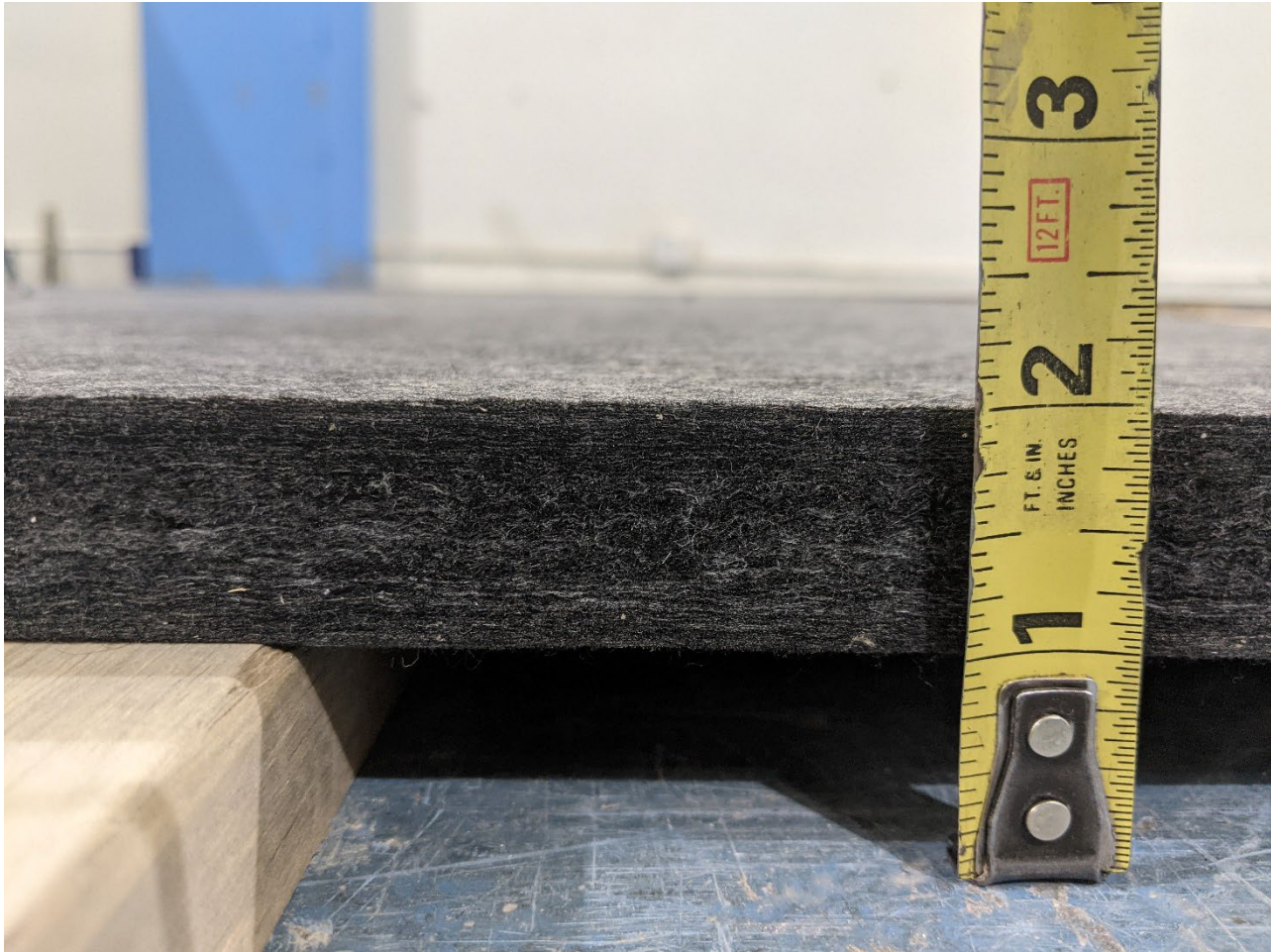
Figure 5 – Detail of specimen materials and airgap depth
