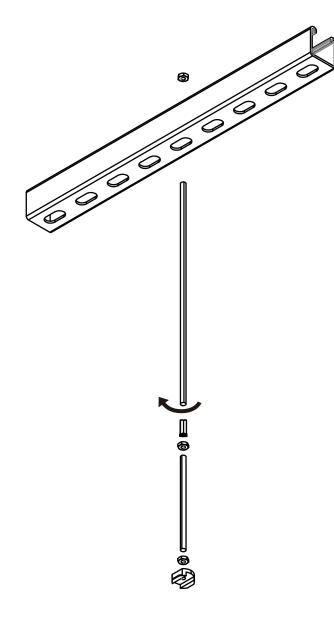
1)Locate the hex coupler for hanger installation positioned at the top side of the luminaire
