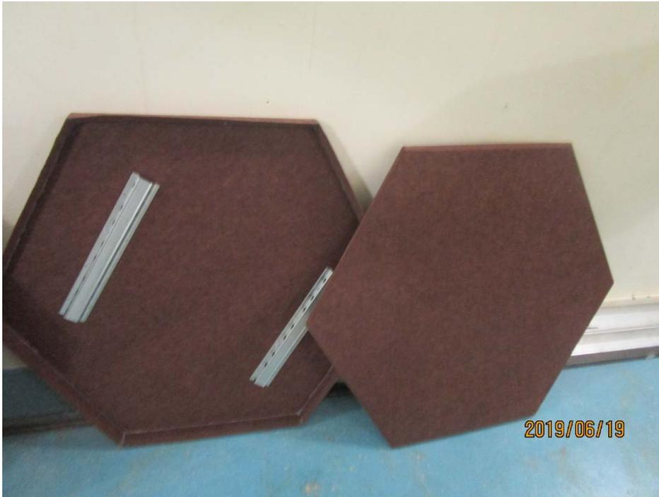
Figure 3 – Body and lid pieces, metal rails at body interior
